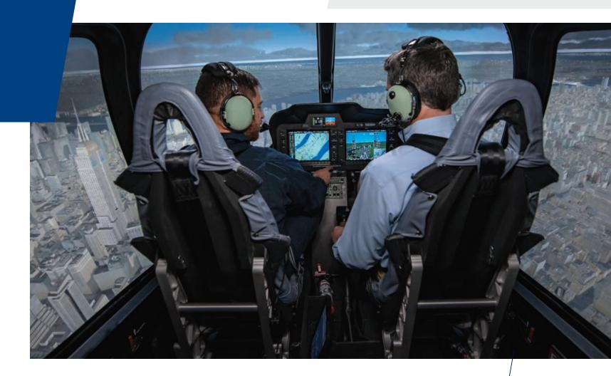
The required components of a Level-D FFS are largely defined by aviation regulators. While these regulations vary from country to country, most are aligned with the FAA (14 CFR Part 60) or EASA (CS-FSTD) which are similar in their requirements. Odyssey Horizon™ simulators meet or exceed all regulatory requirements, but instead of a one-size-fits-all approach like many other simulator manufacturers, TRU Simulation™ prides itself on customizing the training device to meet your specific needs.
