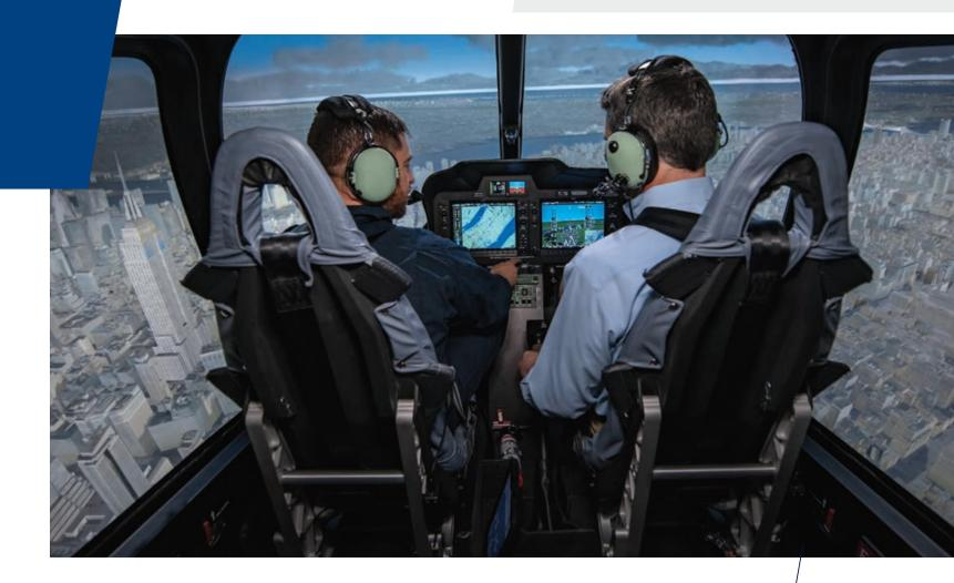
The required components of an FTD are largely defined by aviation regulators. While these regulations vary from country to country, most are aligned with the FAA (14 CFR Part 60) or EASA (CS-FSTD) which are similar in their requirements. Integra Horizon™ simulators meet or exceed all regulatory requirements, but instead of a onesize-fits-all approach like many other simulator manufacturers, TRU Simulation™ prides itself on customizing the training device to meet the customer's specific needs.
